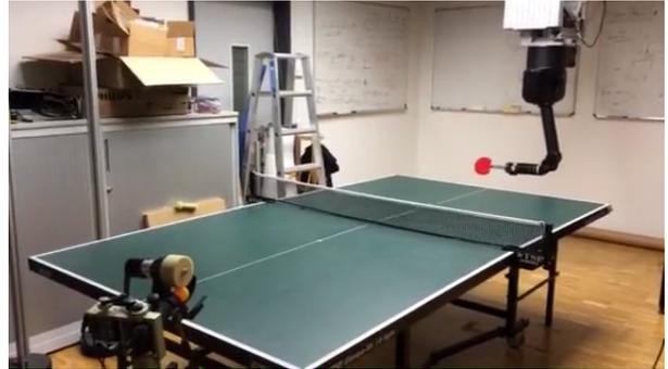
Fig. 1: Robotic table tennis setup with the ball-launcher throwing balls to the robot. In order to hit the ball to a desired position on the opponent’s court, we give the robot reference trajectories that facilitate the right striking motion. We can teach the robot such trajectories via kinesthetic teach-in.
